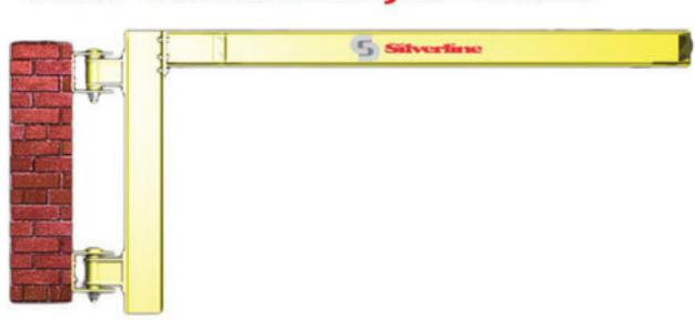
The Wall Cantilever jib crane provides hoist coverage and 200° rotation for individual use, or as a supplement to an overhead crane or monorail system. This jib crane has the advantage of providing maximum lift for the hoist, since it can be installed very close to the underside of the lowest ceiling obstruction.
