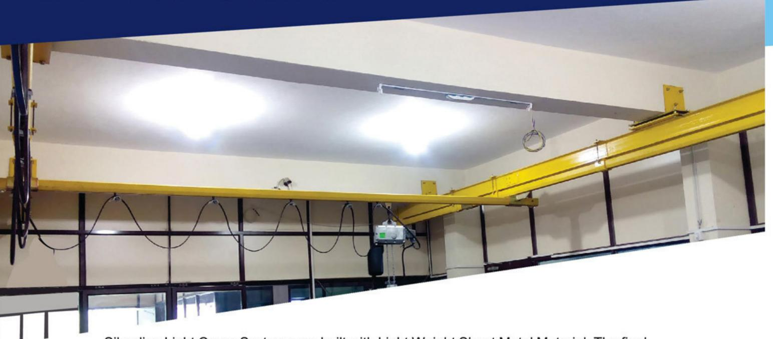
Silverline Light Crane Systems are built with Light Weight Sheet Metal Material. The final Designed Profile is strong enough to carry load upto 2000 Kgs . The Structure can be designed to suit the Shop Or Standard Design can be from Silverline . These Profiles can be Bolted in position and no Welding is required on site. This section can be bend to Achieve Small Turning Radius.
