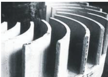
Ventilator guide blades made of VAUTID wear plates VAUTID 100
