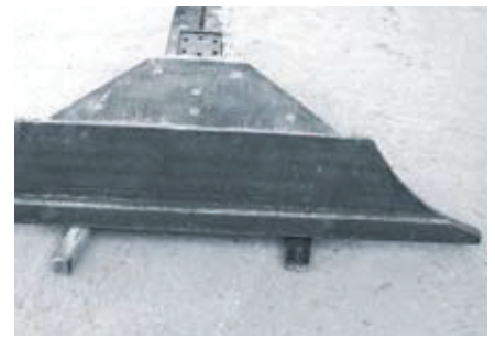
Coke slider for transportation of red heat coke made of VAUTID 145
