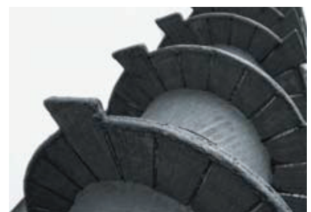
Screw conveyor for waste treatment made of VAUTID wear plates VAUTID 100
