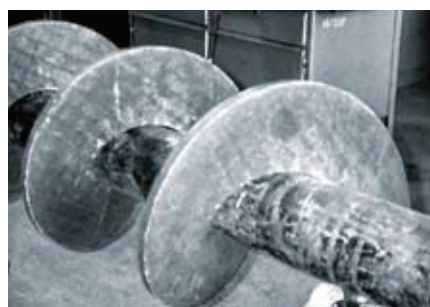
Auger blades of the screw conveyor made of VAUTID wear plates VAUTID 143
