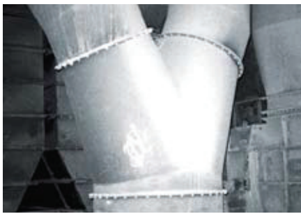
V-Pipe for cement transportation made of VAUTID wear plates VAUTID 100
