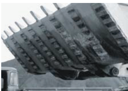
Dredging shovel elements made of VAUTID wear strips VAUTID 100
